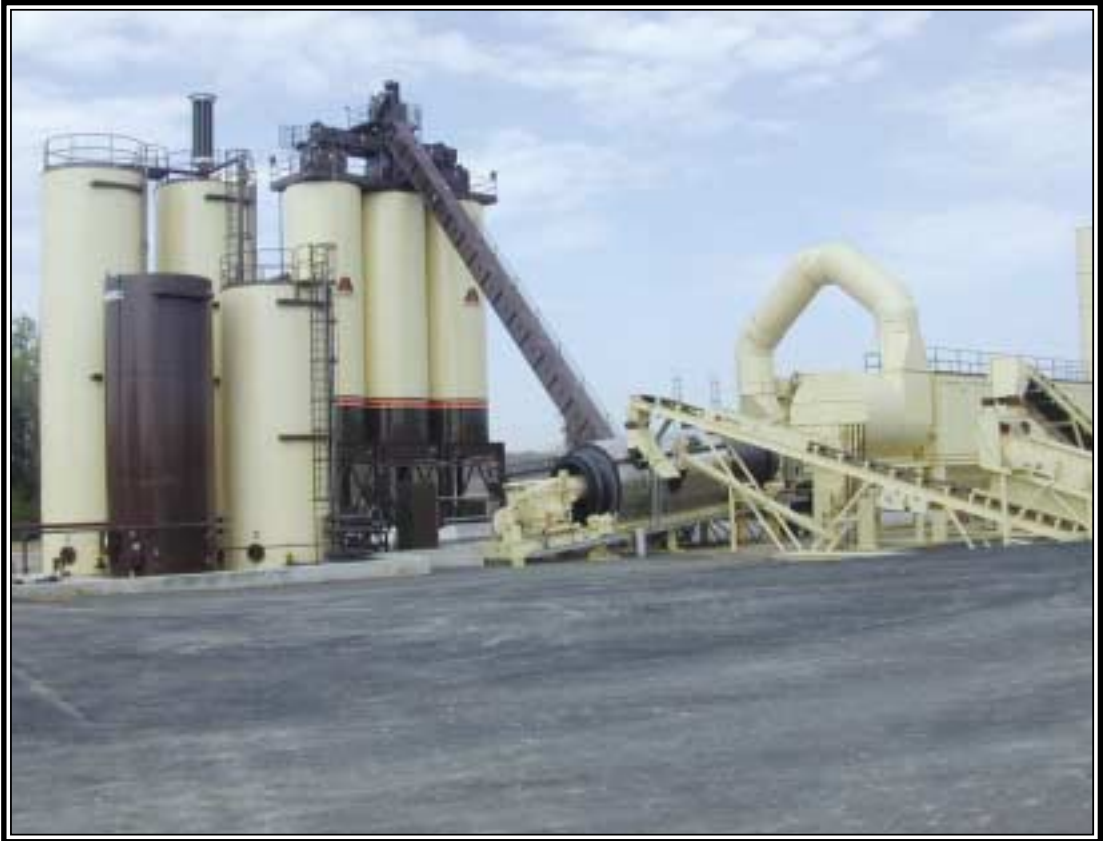
New 400 ton per hour portable Astec Double Barrel Plant with vertical oil tanks and 900 tons of HMA capacity.
